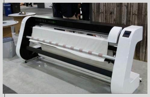
Plotters are used primarily in technical drawing and CAD applications, where they have the advantage of working on very large paper sizes while maintaining high resolution. Another use has been found by replacing the pen with a cutter, and in this form plotters can be found in many garment and sign shops.
