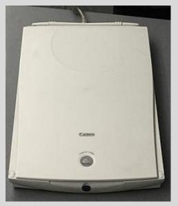
An image scanner—often abbreviated to just scanner—is a device that optically scans images, printed text, handwriting or an object and converts it to a digital image. Commonly used in offices are variations of the desktop flatbed scanner where the document is placed on a glass window for scanning.
