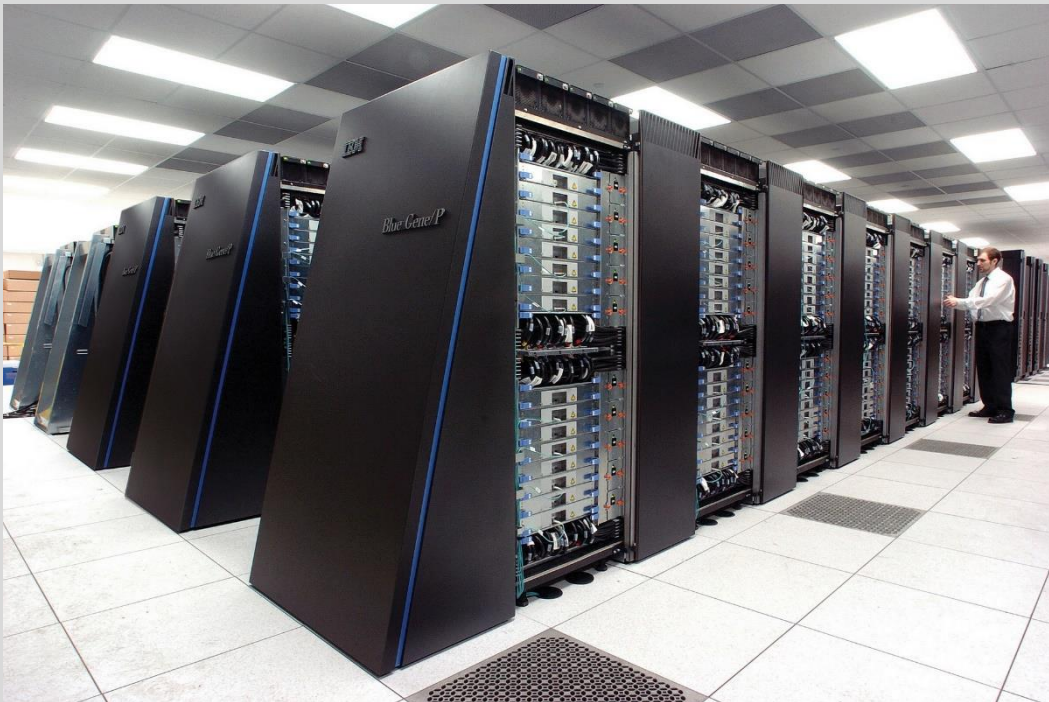
The IBM Blue Gene/P supercomputer "Intrepid" at Argonne National Laboratory runs 164,000 processor cores
